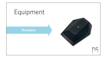
The boundary microphone, like its name, is mounted to a surface, like a wall or a table. You may have seen one in a conference room. The parallel set up of a boundary mic allows it to collect sounds that are reflected on the boundary it is located on.
