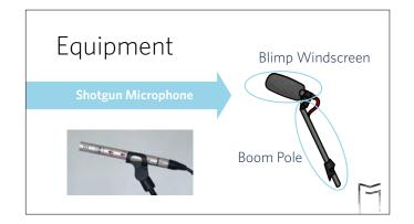
They are highly directional and must be targeted directly towards the sound source which is why a shot gun microphone usually comes with a blimp windscreen, and a boom pole. The operator needs to be careful when holding the mic because small movements can be captured, which can make the sound go in and out in waves.
